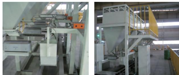
Accurate inoculant feeding by electromagnetic feeder and load cell.
