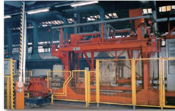
Fully automated pouring for ladle capacity up to five tons.
