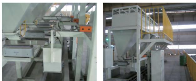
Accurate inoculant feeding by electromagnetic feeder and load cell.
