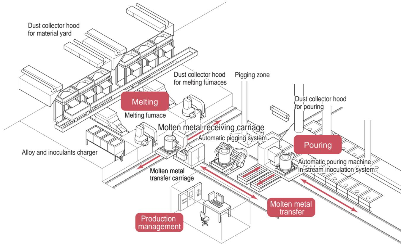
Transfers molten metal safely from melting furnace to pouring area.
