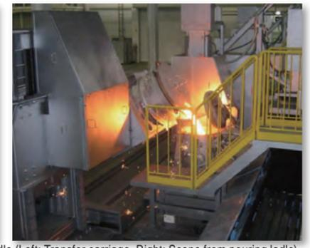
Molten metal is transferred from the transfer carriage into the pouring ladle. This method assures alloy reaction and enables accurate molten metal composition control.
