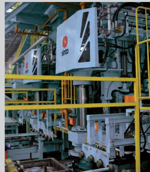
Twin type ACE (Front: Cope molding, Opposite: Drag molding)
