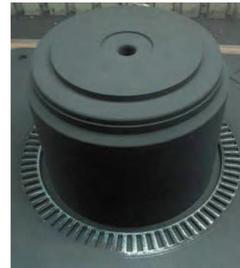
Mold example: Brake drum, φ approx. 500mm
